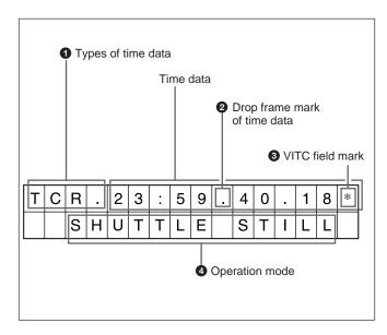
When basic menu item 005 of the setup menu DISPLAY INFORMATION SELECT is set as anything other than OFF, the video signal output from the COMPOSITE (SUPER) output connector, SDI (SUPER) output connector (for J-10SDI/30SDI only) or LOV connector contains superimposed character information (overlaid display), including time code, menu settings, or alarm messages.
