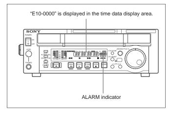
If this happens, the drum and capstan motors stop and the cassette is automatically ejected. Then, the drum starts to rotate again to dry its surface. In this state, the unit is not operable. When the moisture has evaporated, the ALARM indicator goes off and the "E10-0000" message disappears.
