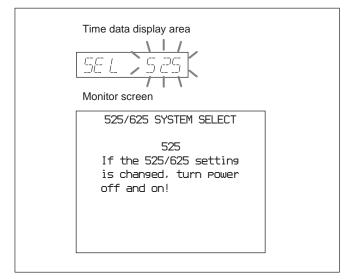
4 Holding down the JOG/SHUTTLE button, turn the JOG/SHUTTLE dial to change the setting from 525 to 625.
