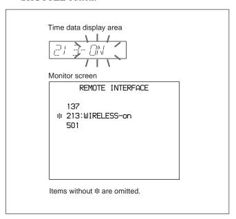
(ON flashes while the JOG/SHUTTLE button is being pressed.)
