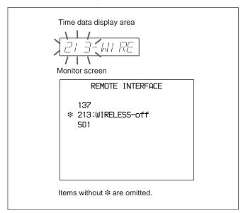
**2** Turn the JOG/SHUTTLE dial to change the setting from "OFF" to "ON" while holding down the JOG/SHUTTLE button, and then release the JOG/SHUTTLE button.
