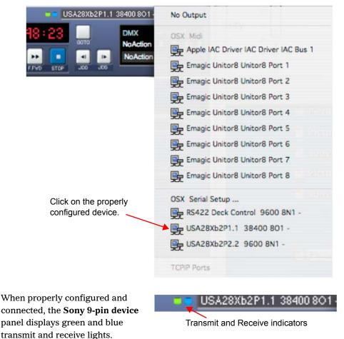
3. Click on the Device field to pop up the menu of devices and click on the properly configured device:
