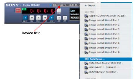
2. Click on OSX Serial Setup... to open the Serial Port Setup window. Select the Sony **9pin38400 baud** preset and click OK to close the window:
