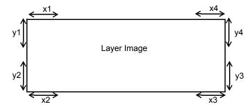
The suggested default DMX value for each parameter is 128, which equals no geometric correction. Values less than 128 move the selected corner left or up; values greater than 128 move it right or down.
