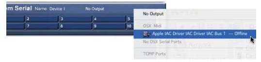
2. When an RS-232 device is attached to one of the PowerMac USB ports, its driver appears in this pop-up menu. By default the menu also includes several PowerMac system options:
