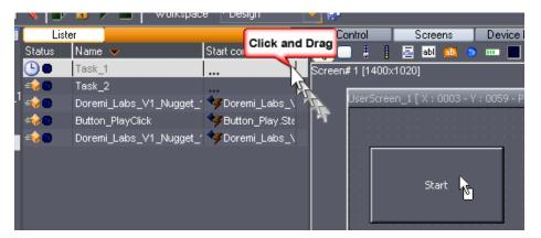
For instance, you wish to start your TimeBased task with a button called "Start". Select "Task\_1" in the Lister and drag it onto "Start" button. The start condition of Task\_1 becomes:
