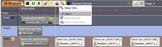
3. A dialog box will ask for the start time of the distribution. When the field has been filled in, press the Spacebar to start the Timeline running.
