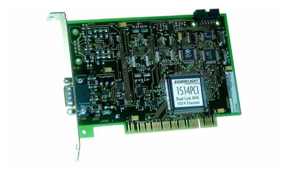
The SoundLight DMX PCI offers up to 1024 DMX input channels or 1024 DMX output channels or combination (512 inputs and 512 outputs). This card handles two complete DMX in/out links in parallel. Up to four cards can be installed in one PC.
