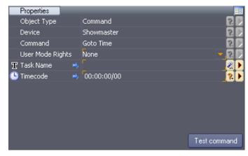
Some properties are constant and cannot be modified. Only properties with orange corners can be changed.
