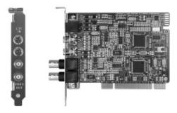
It can either sync to video or freerun with very high precision. The AD RG1 can read and generate LTC simultaneously.
