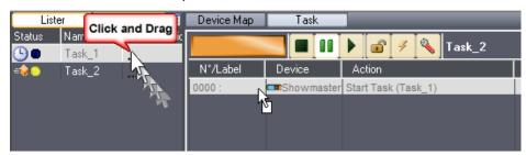
For instance, select Task\_1 in the Lister and drag it into Task\_2 in the Task Editor; a new cue (Start Task(Task\_1)) is inserted.
