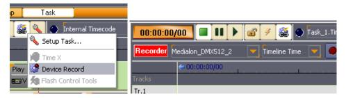
Note that if the device does not support cue recording capability, the Device Record button is not accessible.
