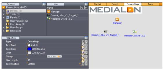
To create a new device, right click inside the tab and select "New Device."
