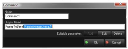
It is important to include any header or ending characters required by the protocol, even though they have been specified in the Frames tab. The settings in the Frames tab only tell the Low Level Communicator MxM how to define the edges of the Frames. Every command must include all bytes to be sent to the device.
