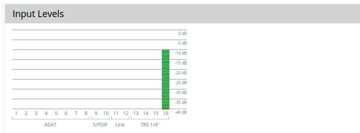
If there are no green bars, try increasing the volume of the audio input. Also see "Planning audio level and latency". For analog inputs you can also increase the input sensitivity.
